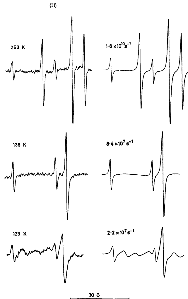
FIGURE 2 Experimental half-e.s.r. spectrum (downfield part) of \text{MeS}-\text{CH}_2-\dot{\text{C}}\text{H}-\text{CH}_2-\text{SMe} (II) at three selected temperatures (left) and computed patterns (right) obtained with the kinetic constants reported. The resulting \Delta G^\ddagger is 2.85 \pm 0.15 kcal \text{mol}^{-1}
